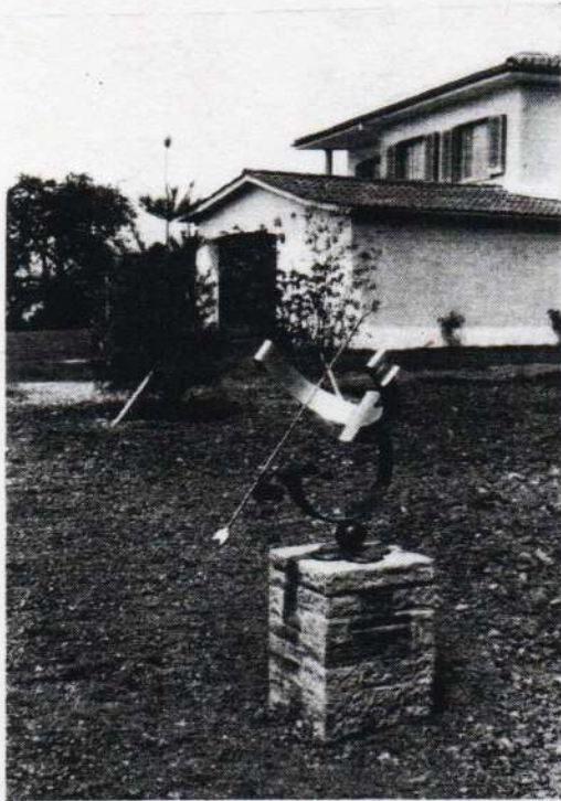
Fig. 8. — Small garden sundial, with equatorial hourdivisions for "mean solar time" on the standard time meridian and time-equation curve. By L.-M. Loske, 1956.
