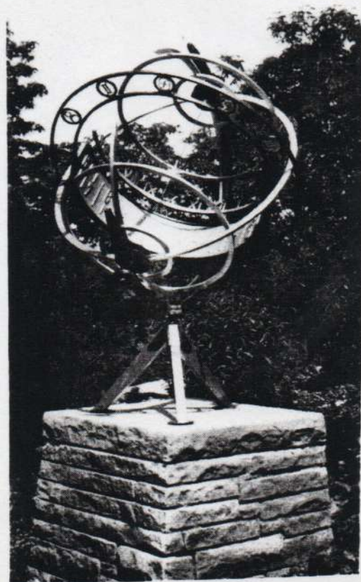
Fig. 7. — Equatorial sundial in a peraluman armillary sphere. De luxe construction with enamelled dial-surfaces, made to the designs of L.-M. Loske, 1956.
