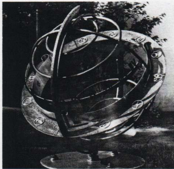
Fig. 4, 5, 6. — Equatorial sundials in wrought iron, made to the designs and calculations of L.-M. Loske, 1954. They belong to various private owners and show "true solar time", "mean solar time", standard time and the solar calendar.
